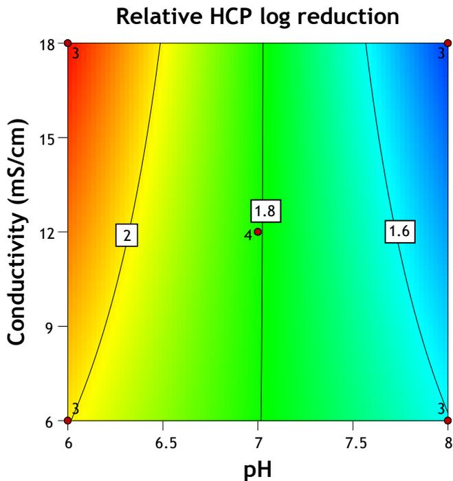
**Figure 5:** Heat map illustrating the impact of various pH and conductivity conditions on HCP removal efficiency for a Vk fragment produced in *E. coli*. The analysis suggests optimal conditions for both HCP reduction and Vk yield represented by the red regions. Sub-optimal conditions are highlighted by the blue regions. These examples demonstrate the importance of optimizing HCPure™ conditions to the specific requirements of each target protein.
